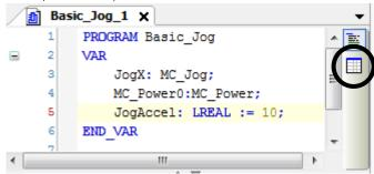
22. To create a new variable, select the "Insert" button in the variable list above the program window.
