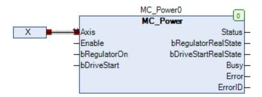
This selects the "X" axis, or rather, the motor connected to the Compax3 is the motor that will be controlled by this function block. NO NEED TO DECLARE "X"! Like our I/O, it's already a "global variable" that is tied to the motor either on our Compax or P-Drive.
