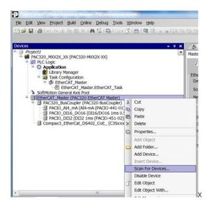
2. A "Scan Devices" dialog box will open showing all the devices available on the EtherCAT network.
