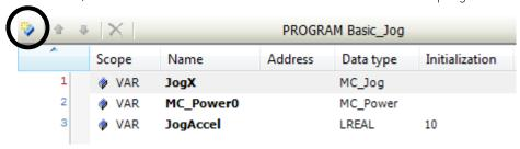
23. Name the new variable "JogVel" and set the initial value to 5. Change the input type to an "LREAL" or a long real.
