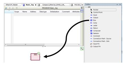
9. Go ahead and start typing "MC\_" a box will automatically pop up with matching functions. Nothing should "MC\_..."
