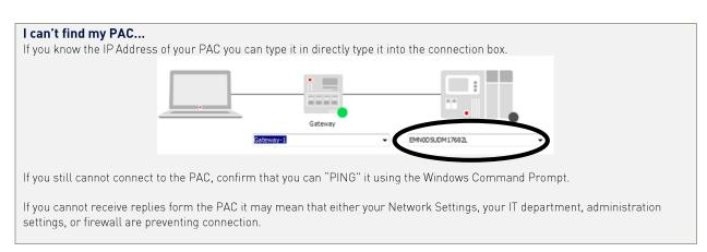
Lastly, the IP address of the PAC may not be what you expect. You can determine the IP address of the PAC by reading it form the SD card. Full instructions on how to do this are in the user manual.
