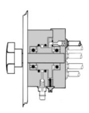
MODEL GV2-10 with 10 outlet ports is shown mounted on an angle bracket attached to machine base.
