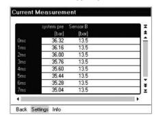
Apart from measurement curves, the HMG 3000 can store userspecific settings (user profiles). The main advantage of this is enabling identical measurements of various equipment items to be repeated for the purpose of preventive maintenance. All the user has to do is retrieve the respective user profile from the HMG 3000's memory.
