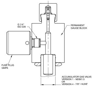
GMP6 Thermal Fuse Plug shown with Permanent Gauge Block for use with a bladder or diaphragm accumulator
