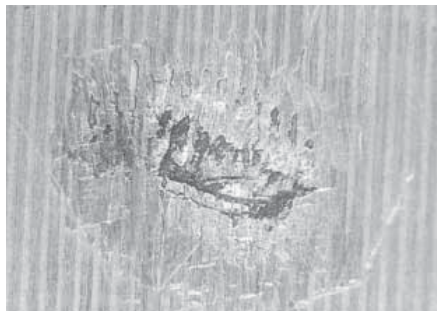
Surface fatigue on ball bearing
