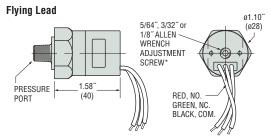
\* Adjustment screw is located under protective screw.
