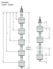
Actuation level distances and  $L_{_0}$  (overall unit length) are measured from inner surfaces of mounting plug or flange. Length Overall ( $L_0$ ) =  $L_1$  + Dimension D. See Mounting Types for Maximum Length values. \*
