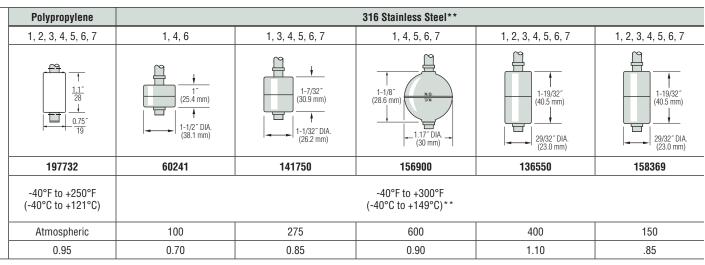
\*\* 316 Stainless Steel floats are available with ceramic potting that allows temperatures to 400°F (204°C); contact factory for these high-temperature applications.
