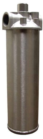
This design has been a standard in the industry for over 40 years. The housing is available in either carbon steel or stainless steel. Maximum operating pressure is 250 psi and standard operating temperature is 275°F. This housing is available with 1" NPT connections only.
