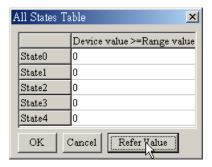
Step 6. "Refer Value" can be used to calculate state range.
