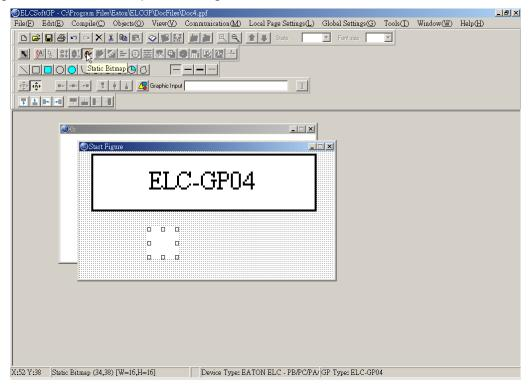
Step 2. In edition display, you can choose static text or static graphics. If you choose static graphics, the mouse pointer will become to cross pointer in the working area. At this time, you can press the left button of mouse and hold on to drag. After releasing the
