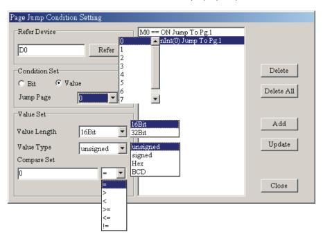
Step 5. After finishing input, press "Add in" to add. The condition will display in the message window. You can press "Update" to update jump page condition or press "Delete", "Delete All" to delete condition.
