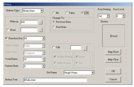
Value: Press this button and GP will display built-in value on screen. You could use function key or common key to enter value. When pressing Enter, GP will send value to ELC corresponding register.
