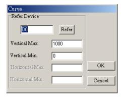
Step 2. User designates D0 device and GP will use D0 content to be sampling points and 100 points max. Odd numbers will be a sets(D1, D3...) and even numbers will be the other sets (D2, D4...). User can use these two sets to draw two curves.
