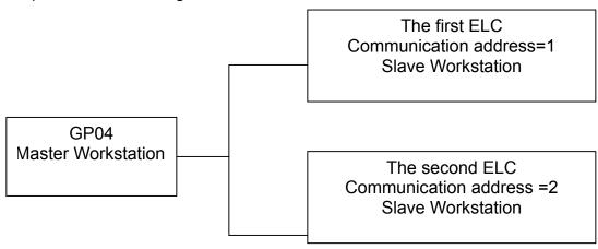
The max. ELC numbers that GP04 can connect is less than 255 ELCs. Master GP connects to slave ELC in series with RS-485. In each ELC, you should give them a different communication address. The setting methods are the same as one-to-one connection but the difference is it needs to set ELC communication address in ELCSoftGP.
