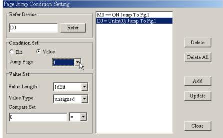
You can set the value length and value type that you need in value setting. Value length could be 16-bit or 32-bit. Value type could be unsigned or signed decimal, hexadecimal or BCD. Condition could be =, <, >, >=, <= or !=.
