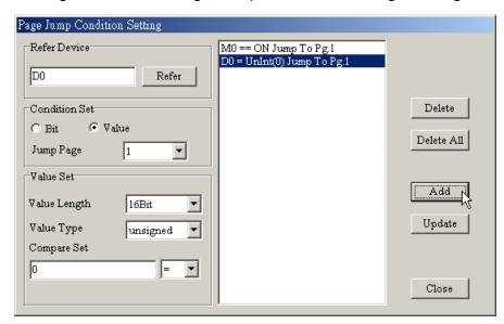
Step 3. Click reference device to input device name, device number and communication address. The devices' name that you can set in this window are X, Y, M, S, D, C and T and the equipment no. are 0~9.
