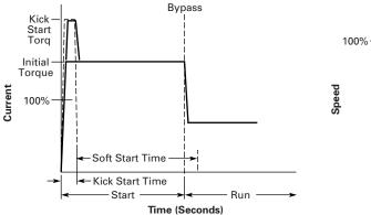
**Note:** Current Limit Starts are not recommended on variable torque load applications like fans and pumps. Attempting starts with the Current Limit set to a value of 20% *Initial Torque* or lower are not recommended as the motor may not develop adequate torque to accelerate properly.
