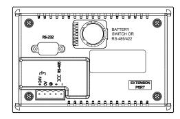
5-PIN terminals: Wire gauge: 12-24 AWG Torque: 4.5 lb.-inch
