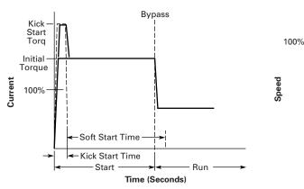
**Note:** Current Limit Starts are not recommended on variable torque load applications like fans and pumps. Attempting starts with the Current Limit set to a value of 20% *Initial Torque* or lower are not recommended as the motor may not develop adequate torque to accelerate properly.
