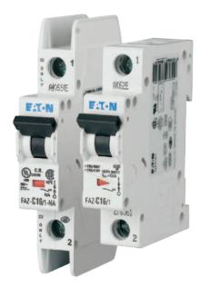
The Eaton series offer two types of miniature circuit breakers for use in North America. The first version, FAZ-NA(RT), fully complies with the molded-case circuit breaker standard UL 489 and the Canadian equivalent CSA 22.2 No. 5-09, which states that devices within that range can be applied legitimately as feeder and branch circuit protective devices per the U.S. and Canadian electrical codes.
