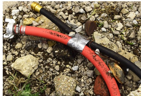
Tape hoses together
