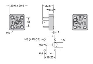
This DIN 43650 Form "A" / ISO 4400, EN175301-803:2000 male connector is specifically designed for mounting in sheet metal. It has an arc over insulating plastic ridge and includes a gasket and four mounting screws. The P10222 connector is designed to mate with Series 5000 or other DIN 43650 Form "A" / ISO 4400, EN175301-803: 2000 female connectors.
