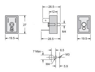
This male DIN 43650 Form "A" / ISO 4400, EN175301-803: 2000 connector can be integrated in tooling to provide a cost effective quick connect electrical interface. The P10020 is designed to mate with Series 5000 or other DIN 43650 Form "A" / ISO 4400, EN175301-803:2000 female electrical connectors.
