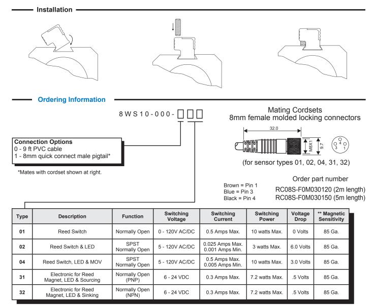
\*\*Minimum gauss rating required for proper operation; as measured 4.5 above sensing surface. Size of sensing area depends upon size and strength of magnet and thickness of cylinder wall.
