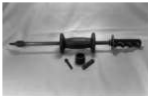
Cam follower removal tool – Removes cam followers with simple tools
