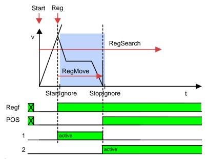
Start Start signal for reg positioning (Steuerwort 1 Bit 4)
