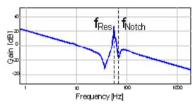
In the Compax3, two notch filters which are independent of each other are implemented.
