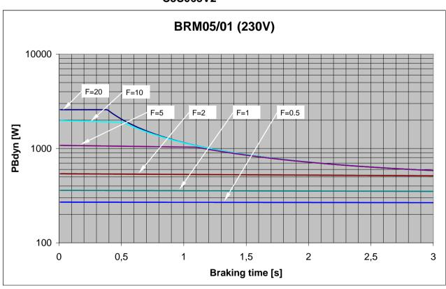
9.4.1.8 Permissible braking pulse power: BRM05/01 with C3S075V4
