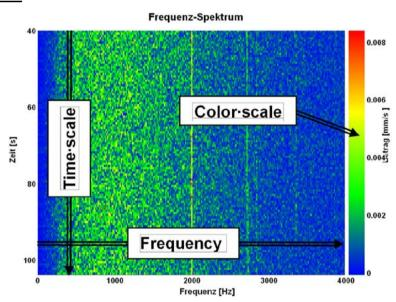
By clicking with the left mouse button on the color scale, you can change between autoscale mode and fixscale mode.
