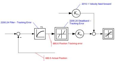
The deadband does no longer supply a velocity setpoint value (zero) for the subordinate velocity loop at small following error. The integrator of the velocity loop stops integrating and the system comes to a standstill.
