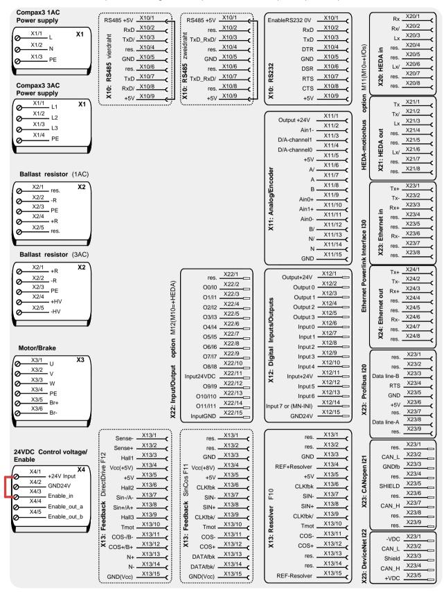
The jumper drawn in at X4 (at the left side in red) is used to enable the device for testing purposes. During operation, the enable input is in most cases switched externally.
