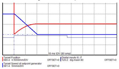
If the homing mode is active, there will always be a homing run with the first start after each configuration download (with the aid of the C3 ServoManager) **Homing run** (see on page 147).
