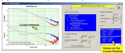
The cursor is set by clicking on the left mouse button. All measurement data of the selected cursor position (frequency) are displayed in the "cursor" operating field.
