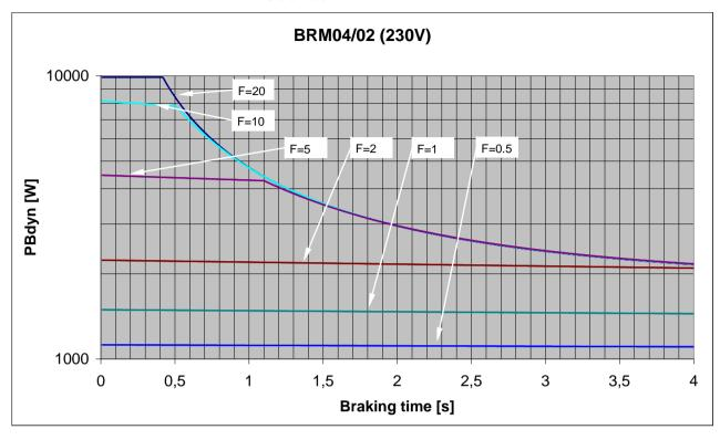
9.4.1.13 Permissible braking pulse power: BRM04/02 with C3S300V4
