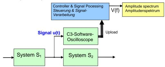
During the spectral analysis of scanned signals with the aid of the discrete Fourier transformation, a so-called frequency resolution (Df) results, Df being =fA/N, independently of the scanning frequency (fA) and of the number of measurement values used (N).
