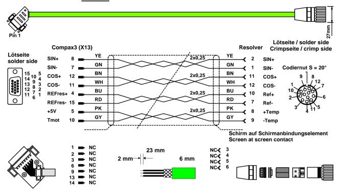
The same cable (with changed conductor coloring) is available under the designation REK41/.. in a version which is suitable for cable chain systems.
