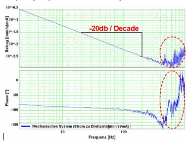
The outlined course at the end of the measurement range does not permit statements on the system measured due to disturbances. Due to the attenuation of the signals increasing with the frequency, the sensitiveness of the measurement to disturbances (signal to noise ratio) increases with a rising frequency. The value as well as the phase response of the displayed frequency response are "disturbed" at the same intensity, this shows, that disturbances are the reason.
