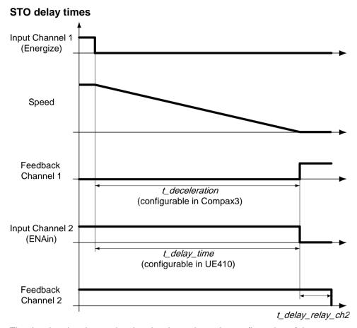
The deceleration time  $t\_deceleration$  depends on the configuration of the Compax3. It must be configured so that oscillation free bringing to standstill is possible, depending on the mechanical load. The delay time  $t\_delay\_time$  must be set in the safety control device UE410 so that  $t\_delay\_time > t\_deceleration$ .
