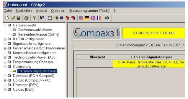
◆ Select the Select the C3 ServoSignalAnalyzer in the function tree under optimization.
