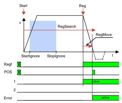
Start Start signal for reg positioning (Steuerwort 1 Bit 4)
