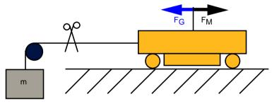
In settled state of the control, the motor force FM corresponds exactly to the load force FG=mxq.
