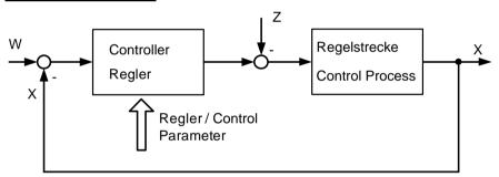
The basic task of a control is the generation and maintaining of a desired state or sequence in spite of interfering disturbances. It is essential that the effects of the disturbances are balanced with the correct force and at the correct time. In the above figure, the setpoint value W represents the desired state and the disturbance value Z represents the interfering disturbance. The actual value X represents the generated and maintained state.
