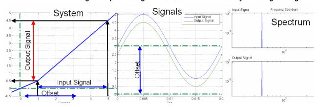
For this, the signal range is shifted so that approximately linear conditions are valid => the results of the measurement show the dynamic behavior at the working point.
