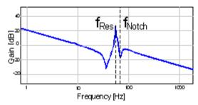
In the Compax3, two notch filters which are independent of each other are implemented.
