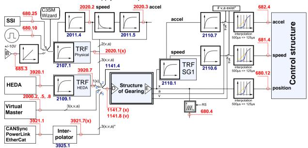
\* Speed v and acceleration a are only present in the event of linear interpolation (bus interpolator: O3925.1) if they are provided by an external source. In quadratic or cubic interpolation, v and a are emulated.
