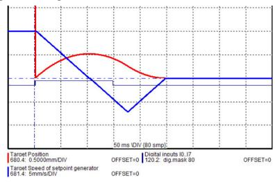
Without positioning after homing run The position reached is not exactly on 0, as the drive brakes when detecting the home and stops:
