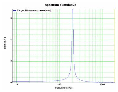
$\Delta f{=}8\text{Hz}$  / f0=204Hz = 25.5· $\Delta f$  / frequency does not correspond to the frequency resolution!
