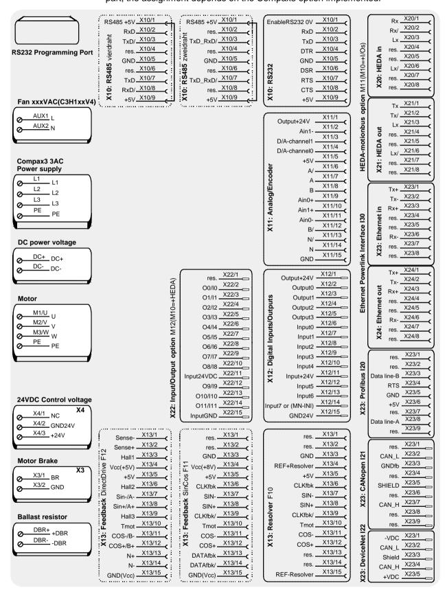
The RS232 programming interface under the upper dummy cover is only available if the X10 jumper at the controller is fitted.
