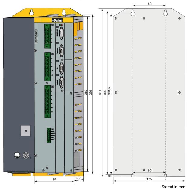
Please respect an appropriate mounting gap in order to ensure sufficient convection:
