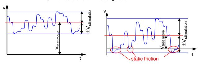
V<sub>test move</sub>: Speed of the test movement V<sub>stimulation</sub>: Speed of the excitation signal
