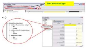
After double clicking on "new", the individual motor parameters are queried by the MotorManager.
