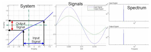
The signal range is reduced so that approximately linear conditions are valid. The results of the measurement will then display the dynamic behavior at the working point.
