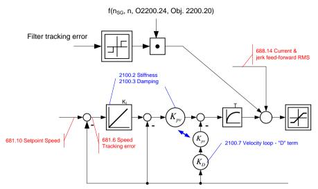
The friction compensation helps the control to surmount static friction at low setpoint speeds. The non linear characteristic line is partly compensated by this and a smaller deadband can be chosen, which will increase the position accuracy. The amplitude of the friction compensation depends on the application and must be calculated if needed. If the value is set too high, corrective movements may result and the tendency to oscillate is increased.
