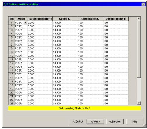
The desired positioning data record is selected via the inputs (I3-I7) and started via a START edge.
