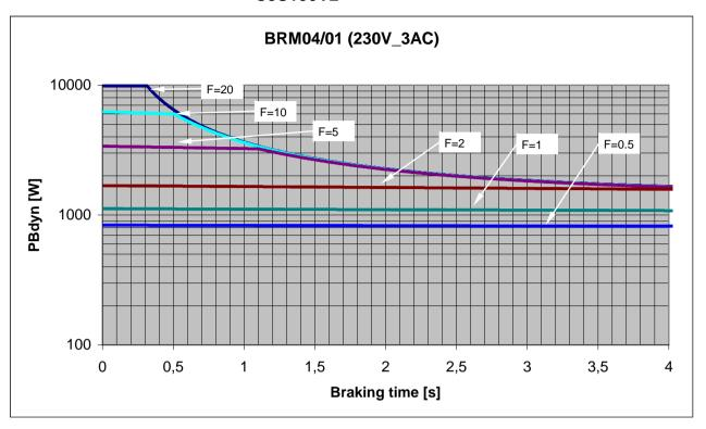
9.4.1.11 Permissible braking pulse power: BRM04/01 with C3S300V4
