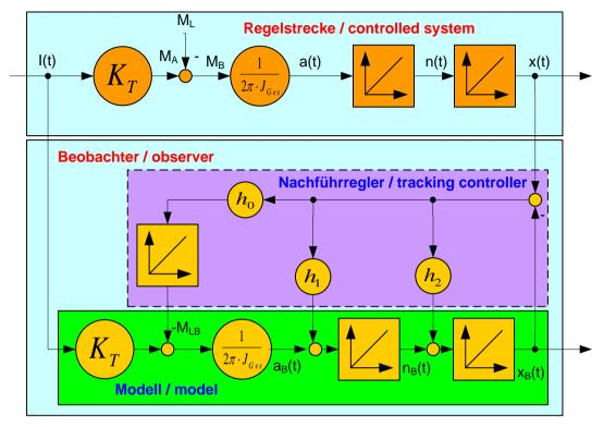
I(t): Torque-forming motor current
