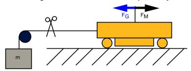
In settled state of the control, the motor force FM corresponds exactly to the load force FG=m×g.
