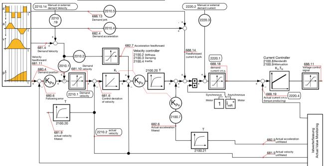
The framed objects are coupling objects for Compax3 - Compax3 coupling via HEDA.
