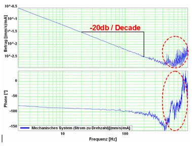
The outlined course at the end of the measurement range does not permit statements on the system measured due to disturbances. Due to the attenuation of the signals increasing with the frequency, the sensitiveness of the measurement to
