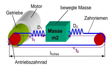
In toothed belt drives, the toothed belt is the elastic coupling element. Its rigidity depends directly on the lengths I1 and I2 and changes in dependence of the position of the moved mass.
