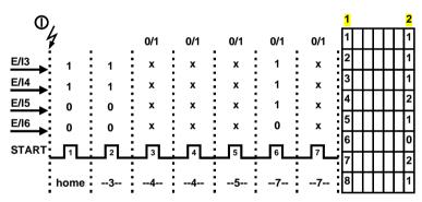
Column 1: Positioning data record address
