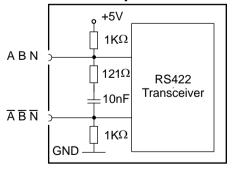
The input connection is available in triple (for A & /A, B & /B, N & /N)
