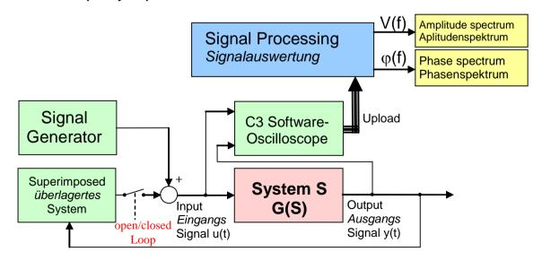
In general, the analysis of the dynamic behavior of a system is made by analyzing the input and output signals.
