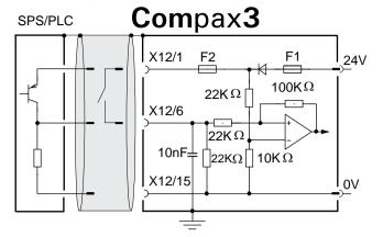
The circuit example is valid for all digital inputs! Signal level:
