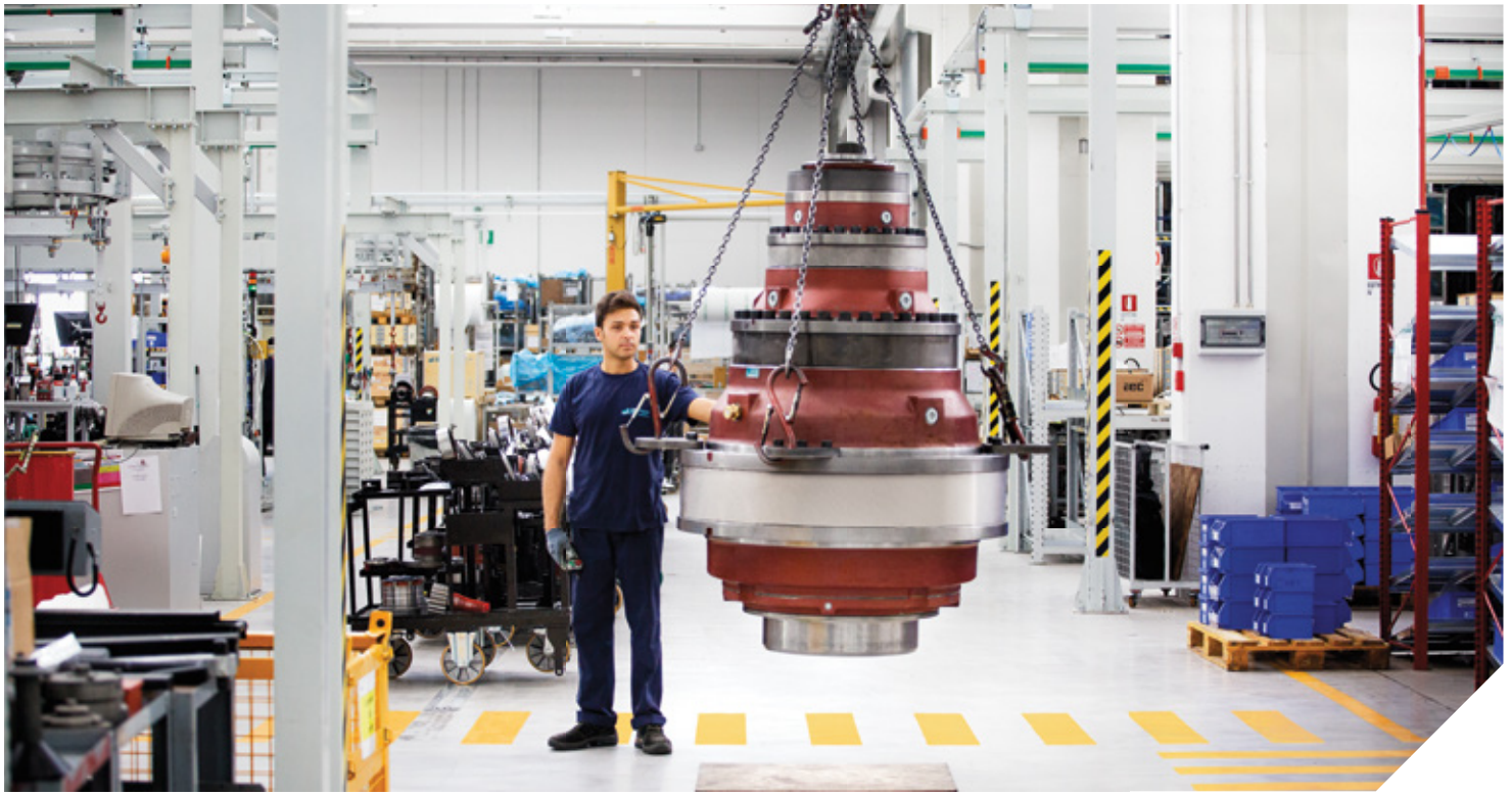
Brevini Power Transmission, Italy: planetary gearbox manufacturing
