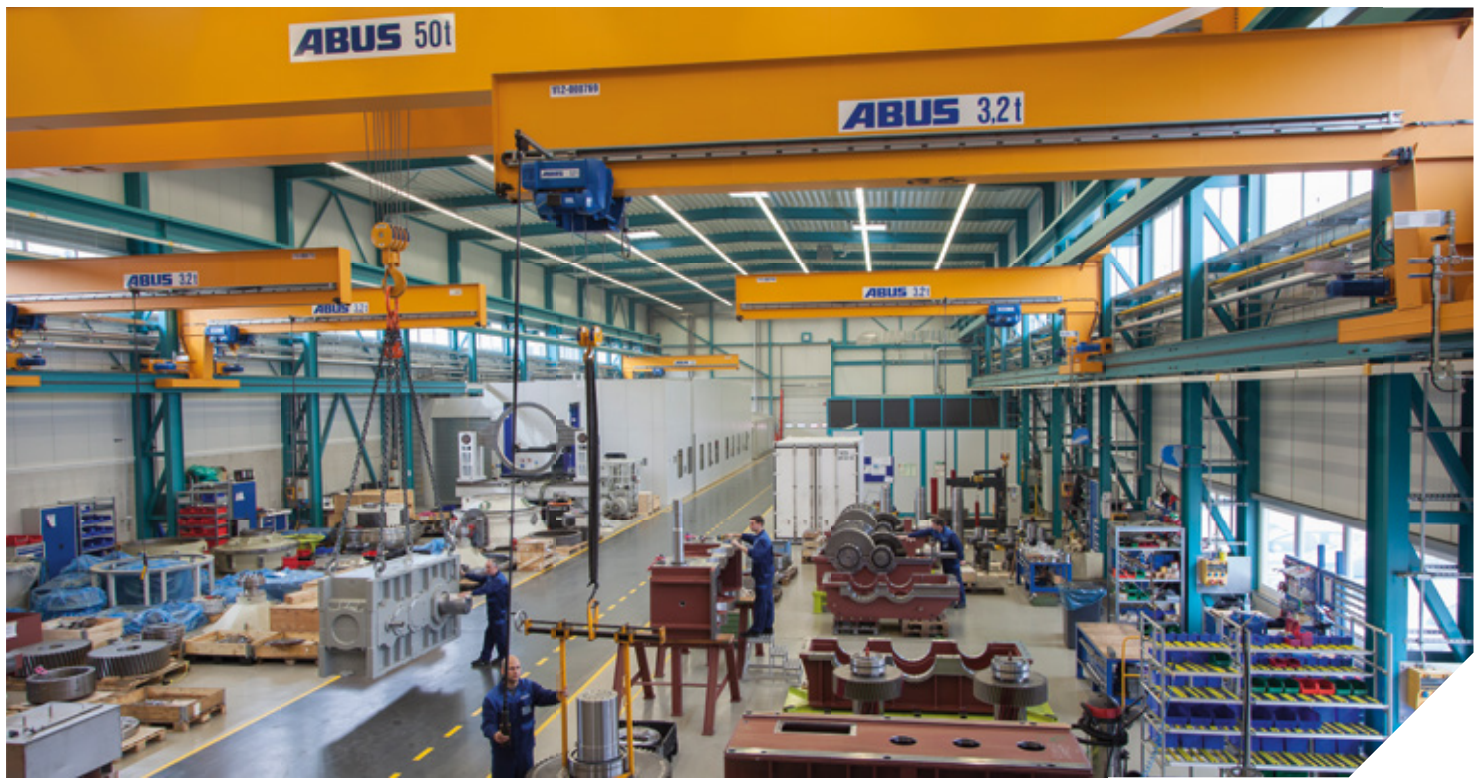
PIV Drives, Germany: hall for assembly of gearboxes up to 40 tonnes
