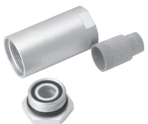
The HIF-Series inline filter is used to protect high-pressure hydraulic systems up to 3,000 PSI. When installed at the pressure side of a pump, the sintered bronze filter element can trap all debris larger than 25um to prevent damage to the valves in the system.
