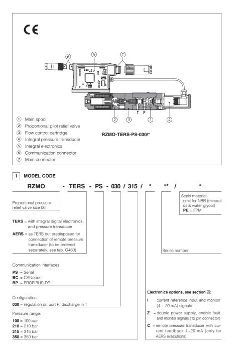
RZMO are spool type proportional pressure relief valves, pilot operated with integral or remote pressure transducer, which provide pressure regulation proportional to electronic reference signals.
