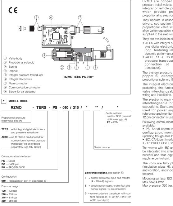
RZMO are poppet type proportional pressure relief valves, direct operated with integral or remote pressure transducer, which provide pressure regulation proportional to electronic reference signals. They operate in association with electronic drivers, see section 2, which supply the proportional valve with proper current to align valve regulation to the reference signal supplied to the electronic driver.
