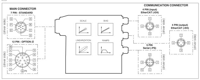
Note: for the electronic connections of 7 or 12 pin main connector, see section 12.1
