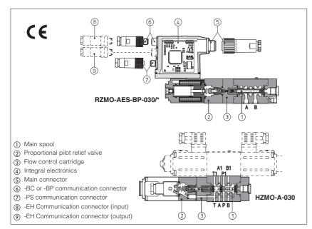
MODEL CODE MO - AES - PS - 030 / 315 / RZ Proportional pressure relief valves size 06 RZ = subplate HZ = modular = without integral transducer Only for RZMO: AE = as A plus integral electronics AES = as A plus integral digital electronics
