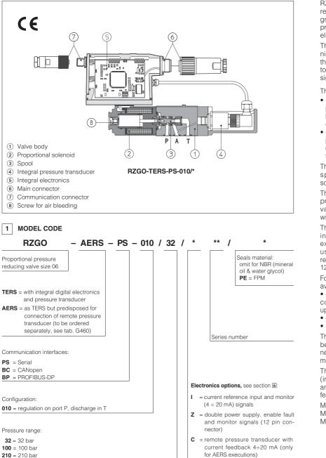
RZGO are 3-way proportional pressure reducing valves, direct operated with integral or remote pressure transducer, which provide pressure regulation proportional to electronic reference signal.
