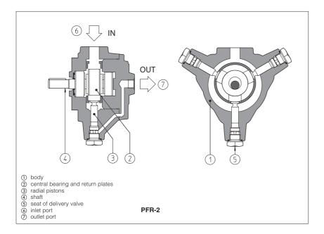
PFR are fixed displacement radial piston pumps with positive drive construction of the pistons 3 (without return spring) for high performance and low noise level.
