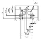
= PRESSURE PORT A, B = USE PORT T = TANK PORT
