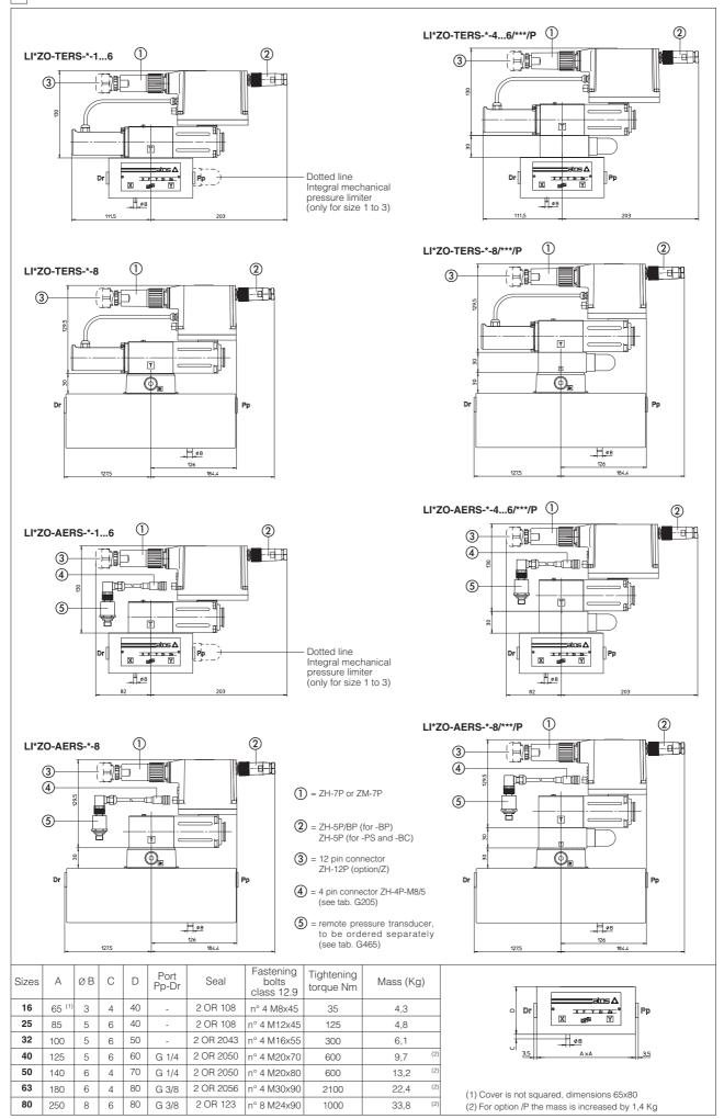
14 COVER INTERFACE AND RECESS DIMENSIONS [mm]
