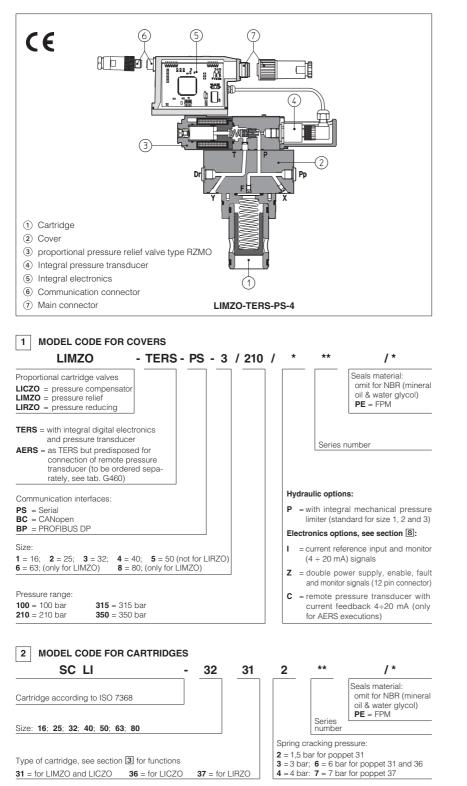
LICZO, LIMZO and LIRZO are 2-way proportional cartridges with integral or remote pressure transducer which respectively provide pressure compensation, relief and reducing controls according to the electronic reference signals.
