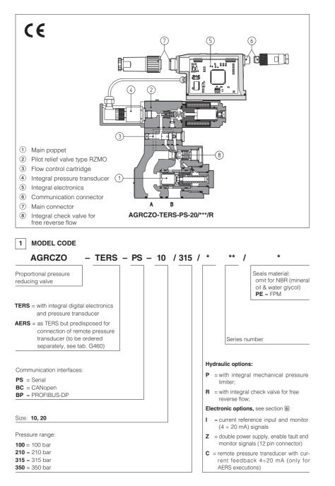
AGRCZO are two-stage normally closed proportional pressure reducing valves with integral or remote pressure transducer wich provide pressure regulation proportional to electronic reference signal.
