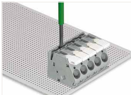
Push jumper bar down firmly using a screwdriver until it hits the backstop – 2706 and 2716 Series.
