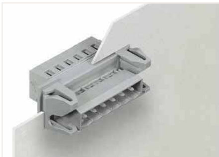
Male connector, with snap-in flanges for feedthrough applications, for 0.5 ... 2.5 mm plate thickness
