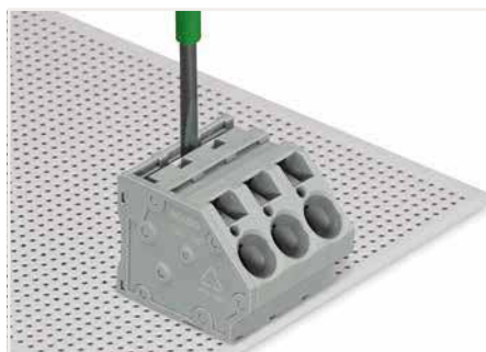
Push jumper bar down firmly using a screwdriver until it hits the backstop – 745 Series.
