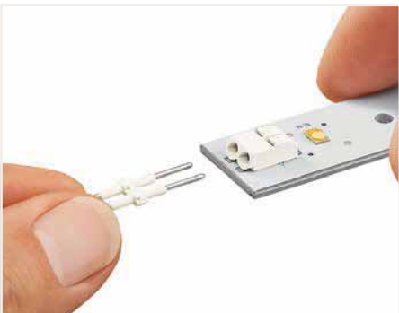
Inserting a board-to-board link into the terminal block.
