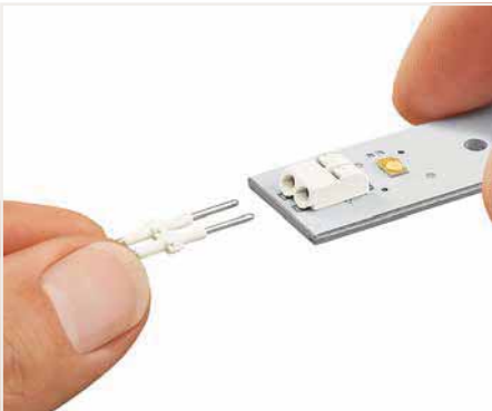
Inserting a board-to-board link into the terminal block.
