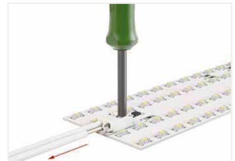
Insert/remove fine-stranded conductors by lightly pressing on push-button (e.g., via 206-860 Operating Tool).
