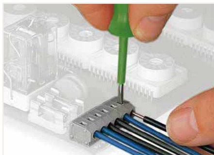
Removing conductor via (2.5 x 0.4) mm screwdriver.
