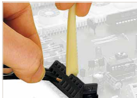
Inserting a conductor via operating tool.
