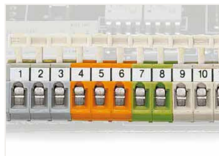
Marking PCB terminal blocks (256 Series).
