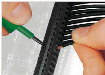
Inserting a conductor via 3.5 mm screwdriver. Screwdriver actuation perpendicular to conductor entry.
