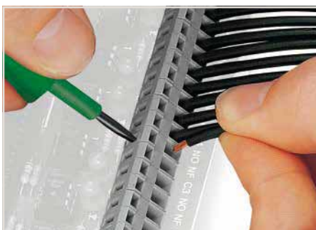
Inserting a conductor via 3.5 mm screwdriver. Screwdriver actuation perpendicular to conductor entry.
