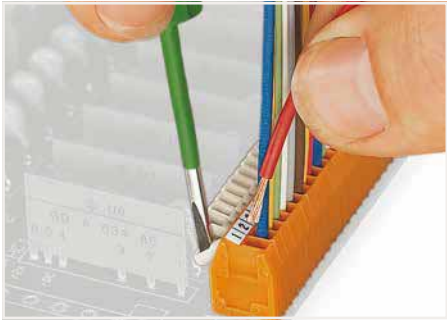
Inserting/removing a conductor.
