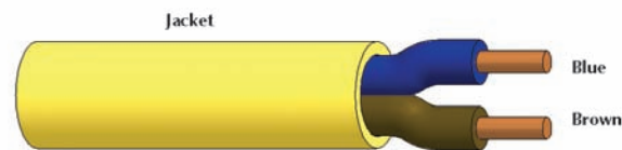
Typical AS-i cable
