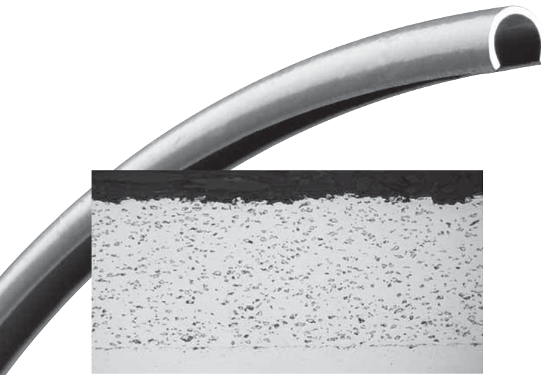
Figure 1: TriCom is a composite coating consisting of a cobalt matrix with chromium-carbide reinforcing phase.
