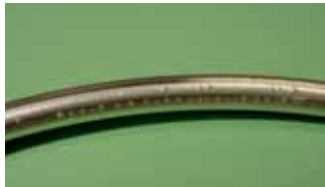
Figure 1: Blisters seen on a standard silver plated seal after 1,000 hours in air at 500°F
