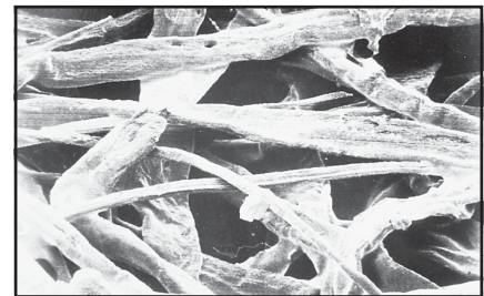
When all mechanisms are combined and utilized by a deep bed of the correct type of filter material, removal of virtually all particles whether liquid or solid, is achieved.
