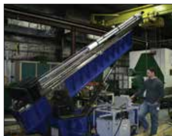
Convertible Test System 20,000 lb load - 100" CC
