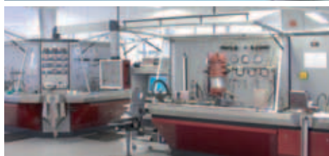
Just one example of the numerous filter testing procedures: Multipass test rig.
