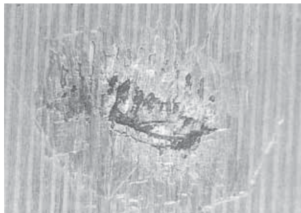
Surface fatigue on ball bearing
