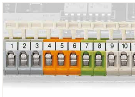
Marking PCB terminal blocks (256 Series).
