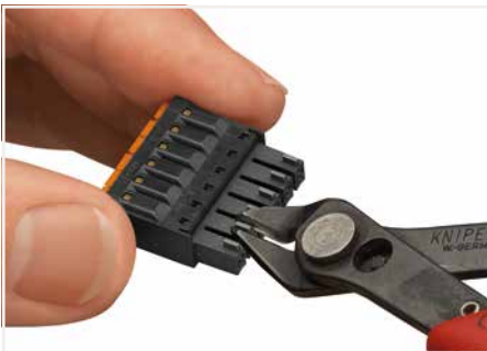
Coding a female connector by removing coding finger(s).
