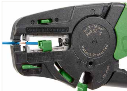
Cutting a conductor.
