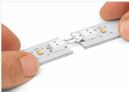
Assembly: Place PCBs on a flat surface and connect terminal blocks on adjoining PCBs via board-to-board link. Disassembly: Pull PCBs apart (max. 10 mating cycles).
