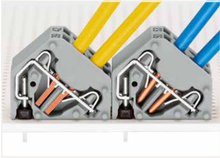
Inserting solid conductors via push-in termination. Inserting/removing fine-stranded conductors: Open the clamping unit using a screwdriver and insert a stripped conductor until it hits backstop.
