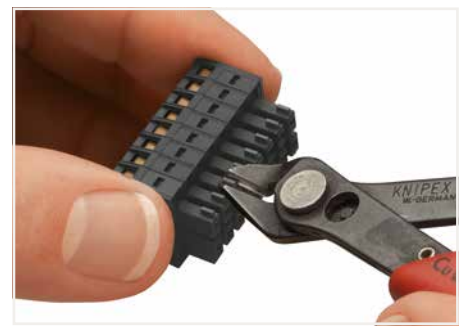
Coding a female connector – removing coding finger(s).
