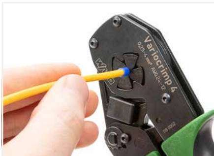
Squeeze handles until ratchet mechanism is released.
