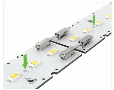
The PCBs must be secured.
