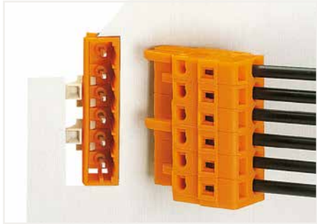
Panel feedthrough male header in large cutout Coding via coding keys: Coding finger(s) opposite to coding key(s) must be broken off.
