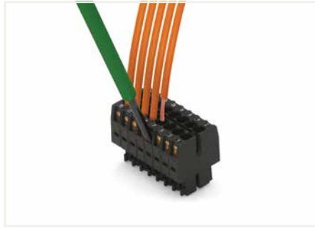
Inserting a conductor via (2.5 x 0.4) mm screwdriver.
