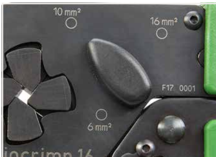
Only for "Variocrimp 16": Adjust conductor cross section with crimping tool in open position.
