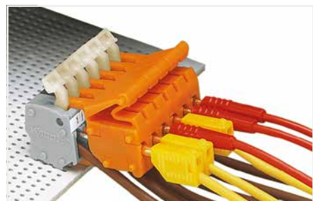
Testing a wired PCB terminal strip.
