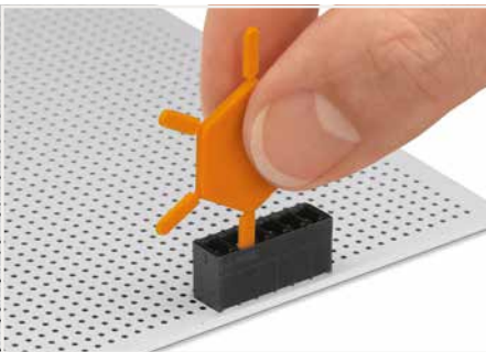
Coding a male header via coding pins.
