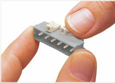
Coding a male header – fitting coding key(s).
