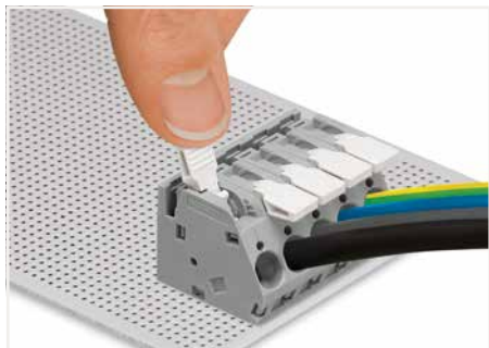
To open the clamping unit, pull the operating lever all the way back – 2706 and 2716 Series.
