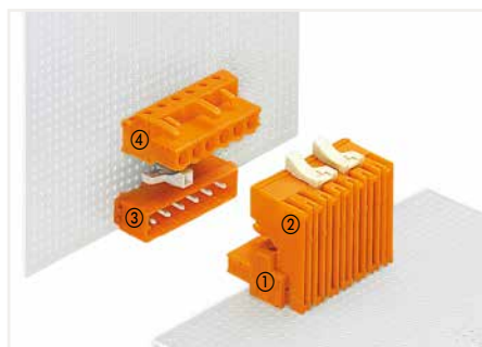
① Female header with angled solder pins ② Male header for double-deck assembly ③ Male header with straight solder pins ④ Female header with straight solder pins
