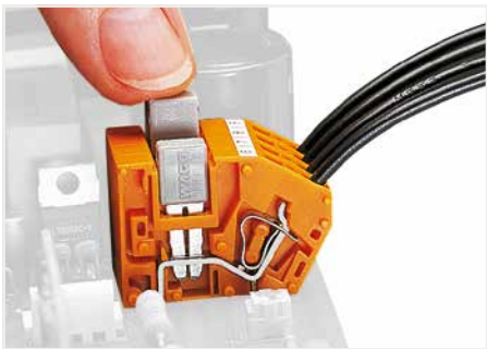
Commoning with adjacent jumpers – push jumpers down until fully inserted.
