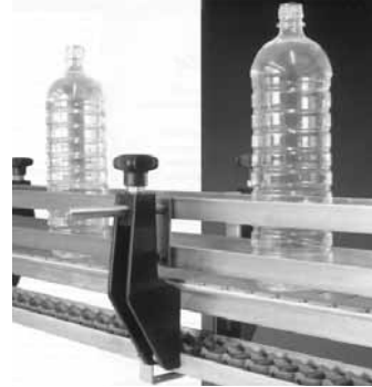
A Capacitive Proximity Sensor “Sees Through” a Wall to Find the Target
