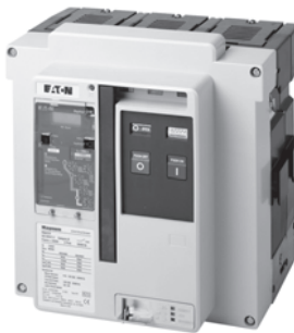
The Magnum MDSX Current Limiting Power Circuit Breakers have fast opening contacts to provide interrupting ratings up to 200 kA at 480 Vac without fuses.
