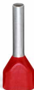
Twin ferrule; Sleeve for 2 x 1 mm 2 / 2 x 18 AWG; red, insulated; 12 mm long
