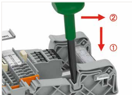
Release the mounting bracket by pushing the operating tool down ① and then forward ②.
