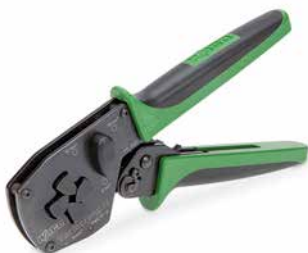
Crimping Tool "Variocrimp 16"; for insulated and uninsulated ferrules; Crimping range: 6 mm 2 (10 AWG), 10 mm 2 (8 AWG) and 16 mm 2 (6 AWG)
