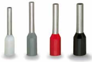
Ferrule; insulated; electro-tin-plated; electrolytic copper; gastight crimped; per DIN 46288 (Part 4/09.09)
