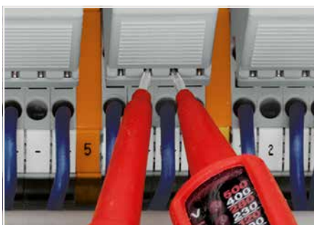
Function testing via touch-proof test slots.
