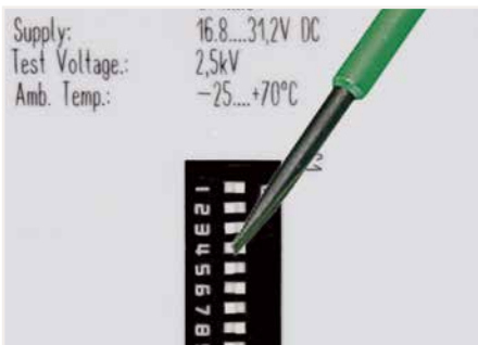
Configuration via DIP switch
