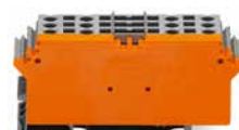
Terminal block for pluggable modules; 12-pole; with 4-conductor terminal blocks; with marker carrier; with orange separator; for 35 x 15 mm and 35 x 7.5 mm DIN-rails; 2.5 mm 2
