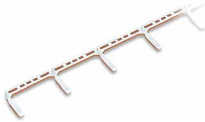
Push-in type jumper bar; 12-way; Nominal current: 16 A; uninsulated
