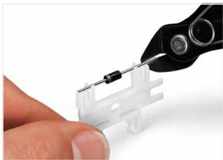
Cutting component to the proper length.
