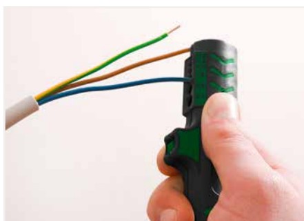
Stripping a wire insulation.
