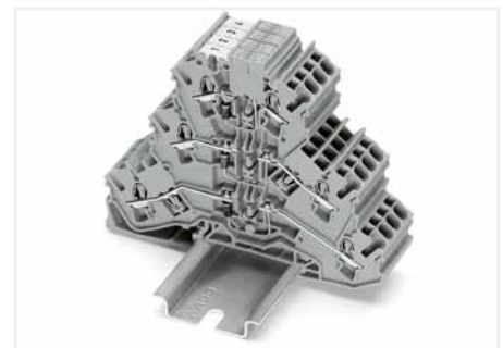
Triple-deck diode terminal blocks were specifically developed for custom diode circuits, such as lamp test and collective fault signal circuits. These terminal blocks provide high-density wiring in a width of just 5.2 mm. Push-in type jumper bars provide additional options for custom circuit design.
