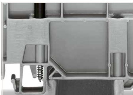
Securing screw – prevents lifting off from the rail. Mounting screw – prevents the cover carrier from being moved on the rail.
