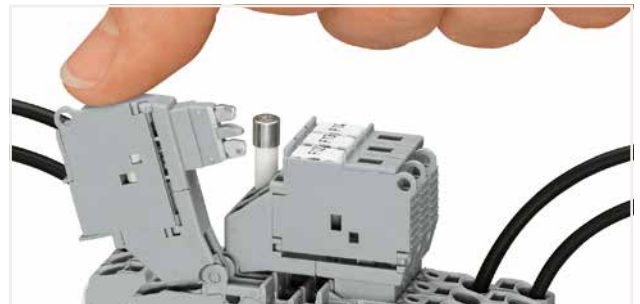
Pivot the fuse holder into the locked open position. Fuse terminal blocks for miniature metric fuses are rated at 2.5 mm 2 (12 AWG) and 6 mm 2 (8 AWG).
