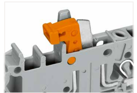
Disconnect/test terminal block with pivoting knife disconnect and mechanical interlock – knife disconnect in open position
