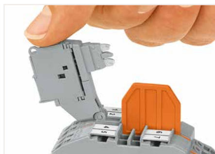
Double-deck fuse disconnect terminal blocks with a pivoting fuse holder (2002-2611, gray) are compatible with disconnect, carrier, through and ground conductor terminal blocks. The fuse holder is also available with a blown fuse LED indicator (e.g., 2002-2611/1000-541 for 12–30 V).
