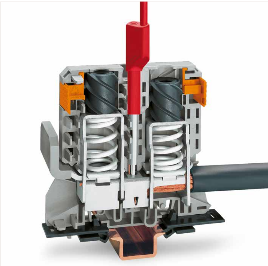
Testing via touch-proof 4 mm Ø test plugs (not available from WAGO, but offered by industry suppliers such as, Multi-Contact Deutschland GmbH).
