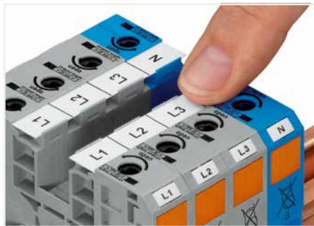
WMB markers or self-adhesive, printable marking strips can be accommodated on 35, 50 and 95 mm 2 high-current terminal blocks.
