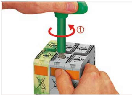
Conductor termination – step 1: Rotate the T-wrench counter-clockwise to the stop ①. Next, push in the orange locking tab. The clamp is locked open for hands-free wiring.
