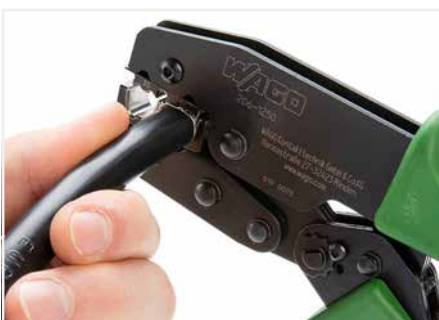
Squeeze handles until ratchet mechanism is released.
