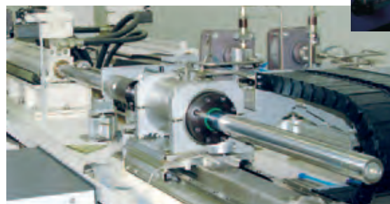
Endurance test rig for hydraulic rod seals – measures friction, leakage and wear of a single seal or sealing system.
