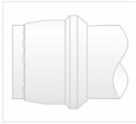
Fig. T47 — Tube not bottomed
