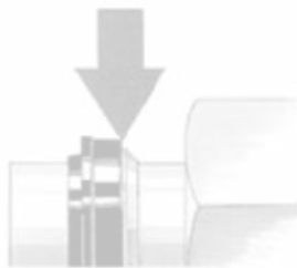
Fig. T50 — Ferrule cocked on tube
