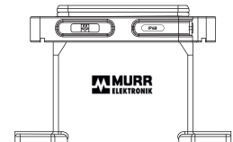
Surface mounted housing Screw locking IP68
