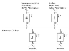
Common DC bus components are used in a multitude of combinations. Drives which are braking can transfer the energy directly to the drives in motoring mode.
