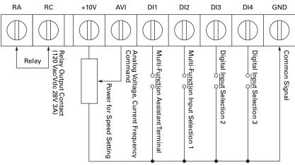
Wire Gauge: 22 – 24 AWG Torque: 4 Kgf-cm
