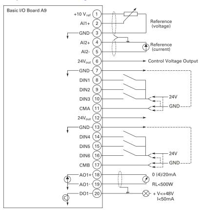
Dotted lines indicate the connections for inverted signals
