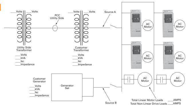
The best way to estimate AFD harmonic contribution to an electrical system is to perform a harmonic analysis based on known system characteristics. The one line in this figure would provide the data to complete the calculations.
