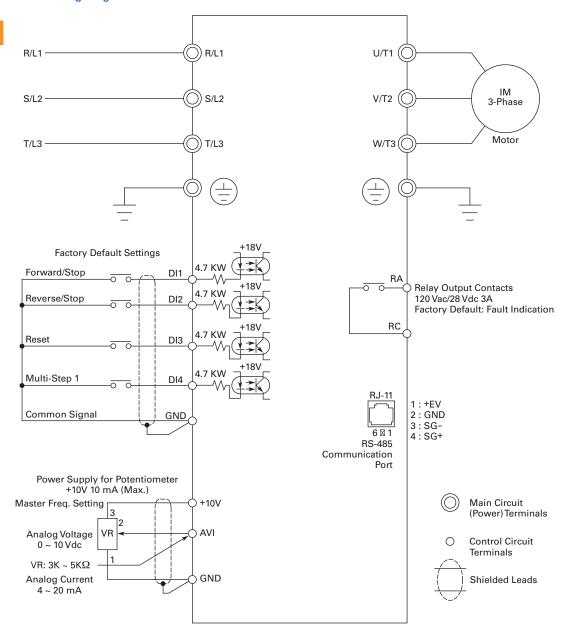
**Note:** Do not plug a modem or telephone line to the RS-485 communication port, permanent damage may result. Terminals 1 and 2 are the power sources for the optional copy keypad and should not be used while using RS-485 communication.
